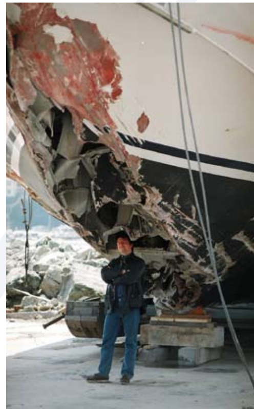
The 30m yacht hit rocks at full speed. A comprehensive, complicated survey of the whole hull structure was necessary as a result of the enormous impact.
