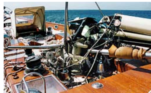
The 38m carbon in-mast furling rig collapsed when the 126ft ketch 'Hetairos' was hundreds of miles off New Zealand.
